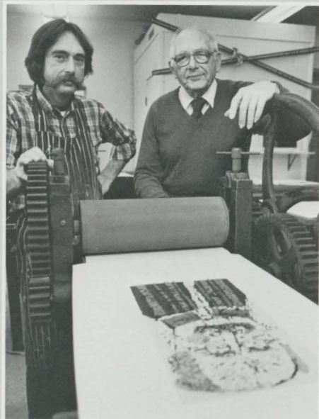
Antique Press Donated — Internationally recognized printmaker and art Professor Misch Kohn (right) has donated his antique Sturges etching press, floor model with book press below, to the art department. Clayton Bailey, department chair, observes Kohn demonstrate the press. Most of Kohn’s works produced during the 1950s and 60s were printed with the press.
