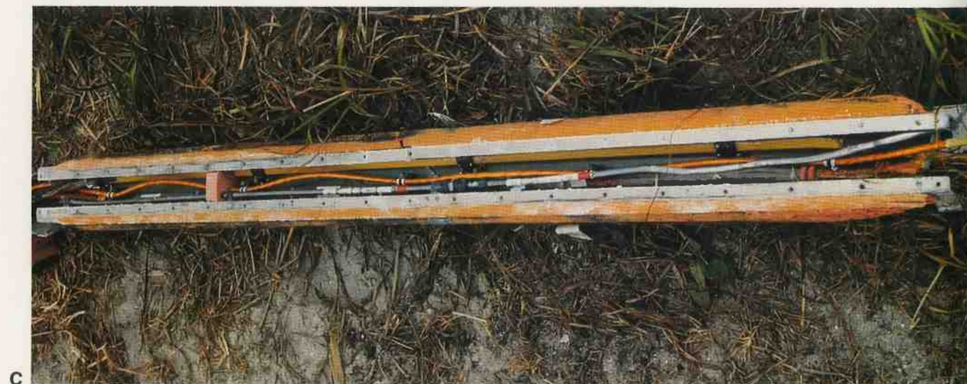
A The upper photos show, from left to right, the left side of the Orbiter (unburned), the right lower and upper rudder speed brake (both burn damaged) and left upper speed brake (unburned), confirmation that the fire was on the right side of the Shuttle stack. The lower photos show the range safety destruct charges in the External Tank. These charges were exonerated when they were recovered intact and undetonated.
