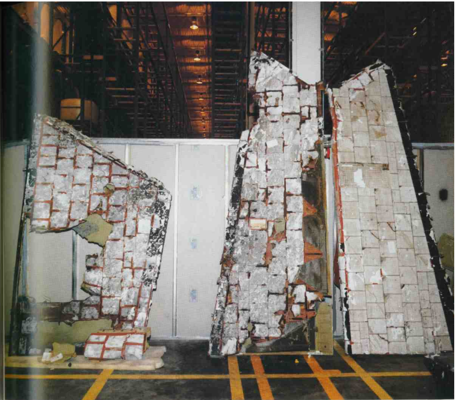
A The upper photos show, from left to right, the left side of the Orbiter (unburned), the right lower and upper rudder speed brake (both burn damaged) and left upper speed brake (unburned), confirmation that the fire was on the right side of the Shuttle stack. The lower photos show the range safety destruct charges in the External Tank. These charges were exonerated when they were recovered intact and undetonated.
