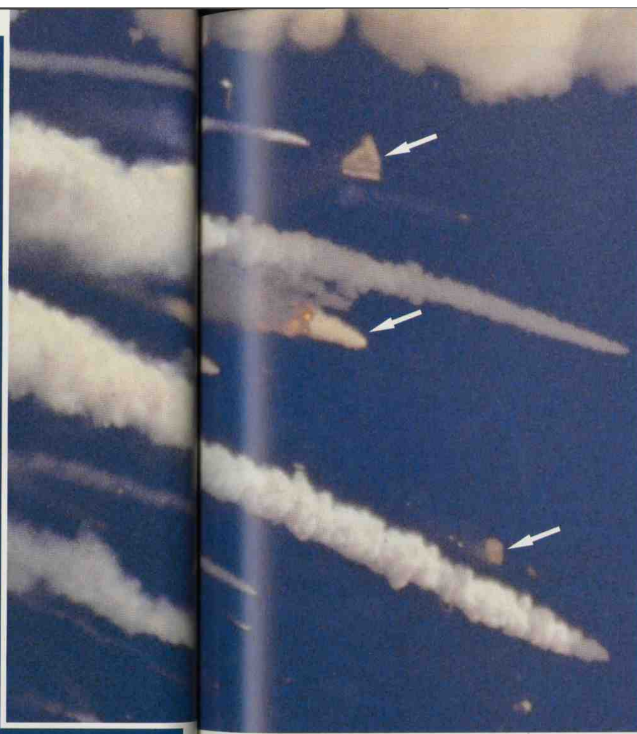
Hurling out of the fireball at 78 seconds (left) are the Orbiter's left wing (top arrow), the main engines (center arrow) and the forward fuselage (bottom arrow). In the photo below, it plunges Earthward, trailed by smoking fragments of Challenger.
