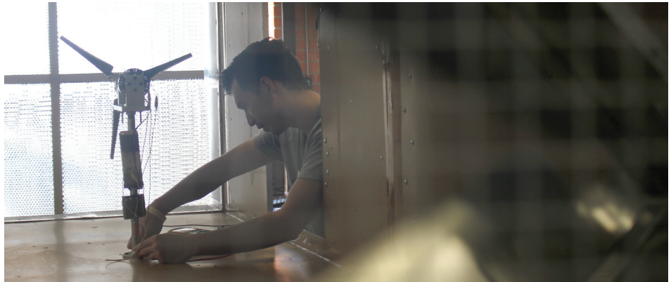
MECHANICAL ENGINEERING STUDENT ALEC SAFRENO PREPARES A WIND TUNNEL FOR A DEMONSTRATION OF THE COLLEGIATE WIND COMPETITION TEAM'S SCALE MODEL TURBINE. THE WIND TUNNEL WAS CONSTRUCTED BY A PREVIOUS CAL MARITIME TEAM THAT PARTICIPATED IN THE SAME COMPETITION.
