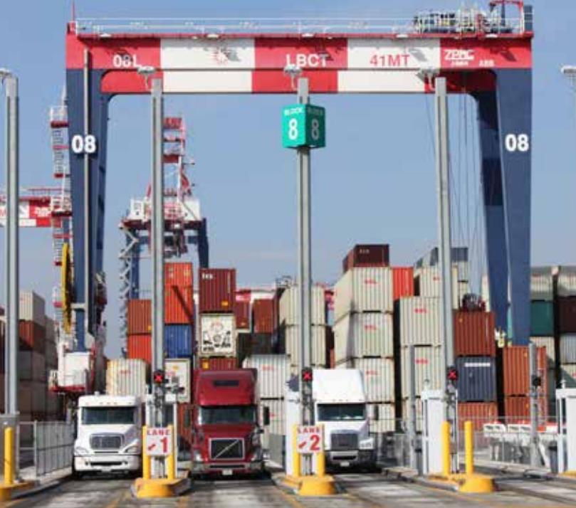
ROBOTS WON'T OPERATE OVER A TRUCK UNLESS THE DRIVER IS OUT OF THE VEHICLE. SENSORS LET THE ROBOT KNOW WHEN THE DRIVER IS CLEAR AND WORK CAN BEGIN.
