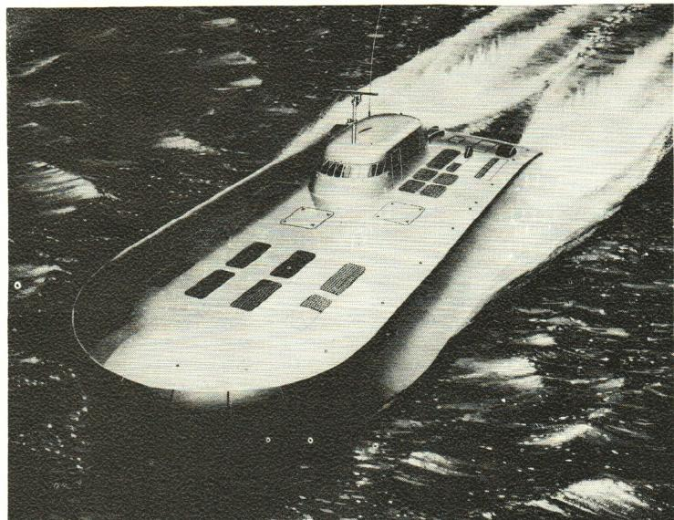
transoceanic transport of 5,000 tons and above. The ship will be capable of crossing the Atlantic in less than two days. It will carry containerized cargo and be highly automated. The craft is a joint venture of Bell, the U.S. Navy and the Maritime Administration. The craft will have solid catamaran-like sidewalls that contain the air bubble upon which it rides. The sidewalls will not permit am-
