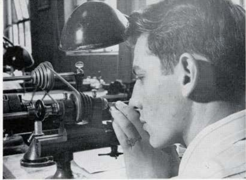
Tom Reasonover is shown above at delicate and precise work in Horology lab — watchmaker's lathe.
