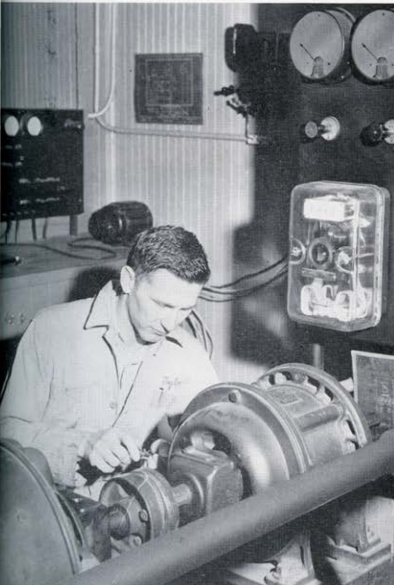
Frank Taylor, senior Industrial Arts major, is demonstrating a motor generator set in the electrical shop.
