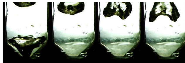
FIGURE 9. Deceleration following exit of air slug (5.56 ms between images)
