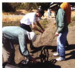
Members of associate professor Mitchell Craig's research team use ground-penetrating radar to take images beneath the surface at the Green Valley fault near Fairfield.
