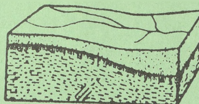
1d Monoclinal fold caused by faulting at depth
