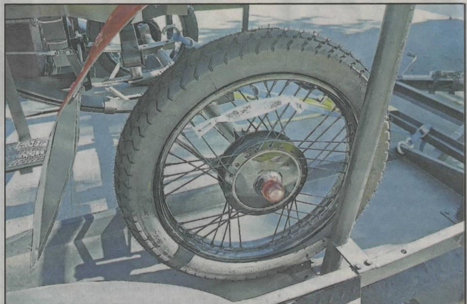
The front wheels of Bob Cryder's 1904 Oldsmobile Pie Wagon are from a Yamaha motorcycle. For many other parts, a local blacksmith shop helped Cryder weld metal into the shapes he needed.
