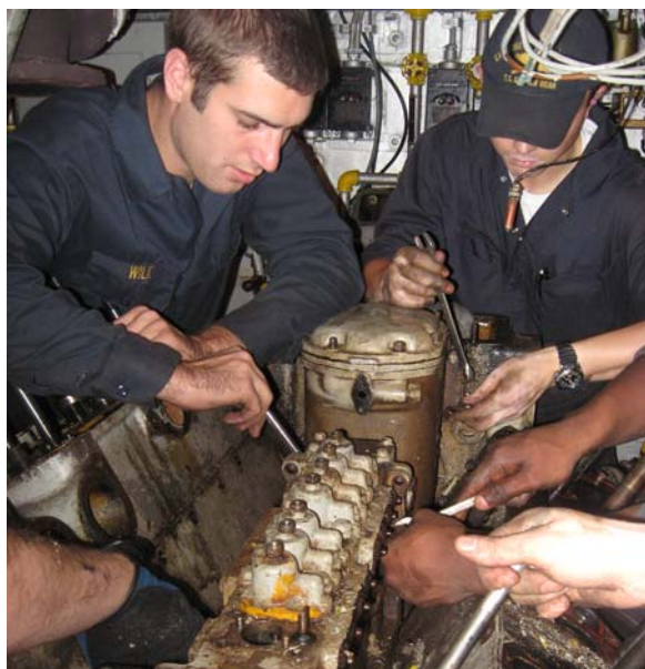
Mike Wilk and Paul Barang concentrate on removal of the fuel pump from the old engine aboard the Cub , while other cadets tackle components along the top of the block. Many hands speed the process while cadets get invaluable experience in the construction and operation of diesel engines.
