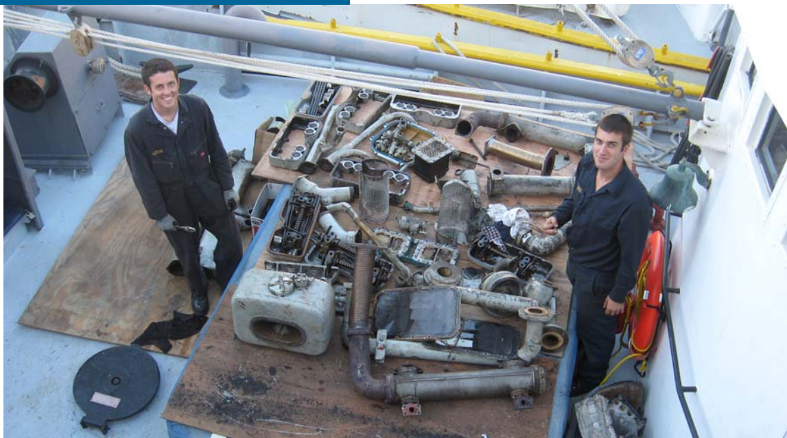
Mike Wilk and Paul Barang concentrate on removal of the fuel pump from the old engine aboard the Cub , while other cadets tackle components along the top of the block. Many hands speed the process while cadets get invaluable experience in the construction and operation of diesel engines.
